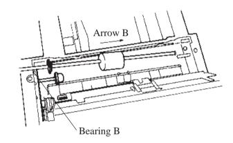
Figure 5.6 Slide the Pick Roller
